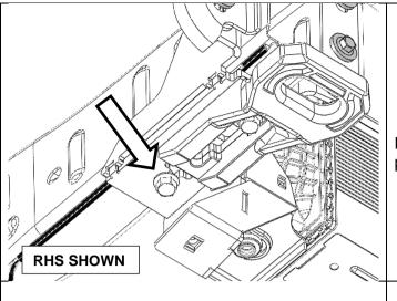
35. Insert the recovery point over the chassis and insert an M12 flange head bolt removed in Step 30 into the rear most hole on the underside of the recovery point.
