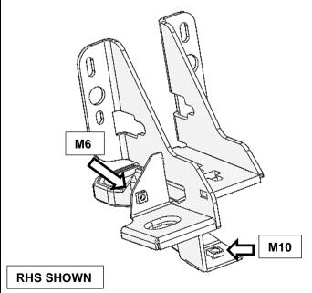
9. Insert M6 and M10 cage nuts into locations shown.
