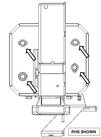
14. Position chassis mount assembly over chassis endplate and insert the supplied four M10x45mm bolts and flange nuts through the mount and recovery point as shown. Do not fully tighten.
