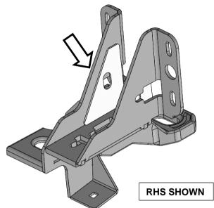
36. Insert two triangular spacer plates on either side of the chassis between the recovery point.
