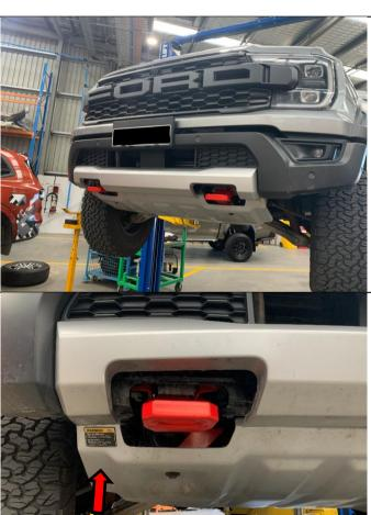
44. Replace removed bumper section, number plate and bash plate removed in Steps 25. 27-28.
