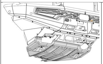
If already installed, remove centre bash plate, wing under panel, and ARB stone guards from bull bar. (Refer to ARB bull bar fitting instructions).
