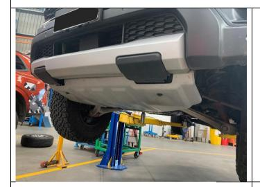
25. Remove bash plate by removing four M10 bolts.
