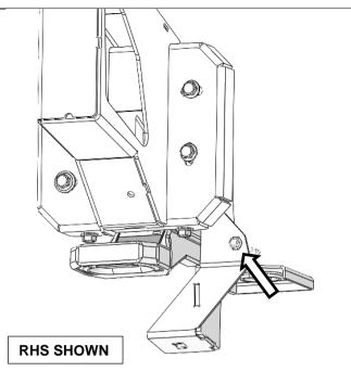
21. Fasten intercooler to recovery point using fastener removed in Step 3.
