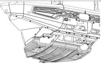
22. Replace all under panels in reverse order to how they were taken off and torque to specification.
