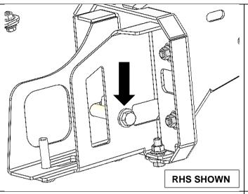
7. Remove M12 through bolt and crush tube, careful not to let the crush tube fall into the chassis.
