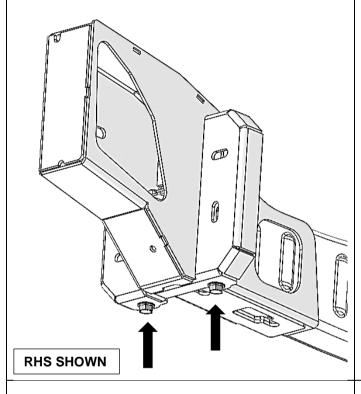
8. Remove the two M10 bolts from the bottom flange of the mount.
