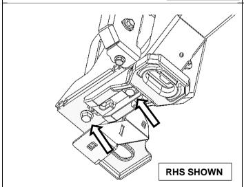
18. Tighten M12 bolts at the base to ensure the recovery point is seated properly against the chassis and then loosen.
