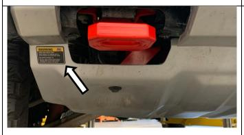
23. Place warning label adjacent in a location that would be visible to the operator. Clean area prior to placing sticker.
