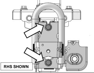
30. Remove both factory tow hooks by removing two M12 bolts.
