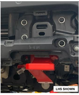
42. Fasten four M10x45 flange head bolts, washers and flange head nuts through the front of the bumper. Torque to required specification.
