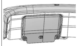
26. Remove tow hook covers by removing two fasteners underneath. Discard removed parts and J-clips.
