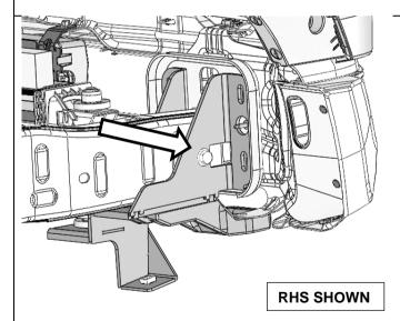
37. Insert the crush tube, M12x110 bolt, washers and nyloc nut through the chassis. Crush tube must be inserted from the inboard side of the chassis.
