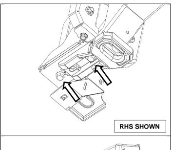
Insert M12x50 fastener supplied with the bull bar through the rear hole in the base into the chassis.
